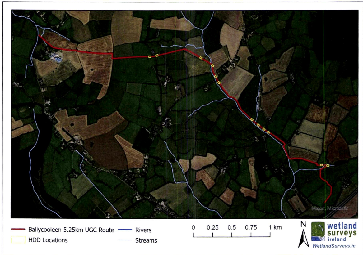
Figure 3: HDD pit locations.
