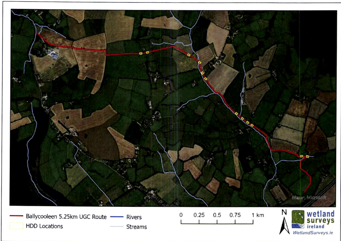
Figure 3: HDD pit locations.
